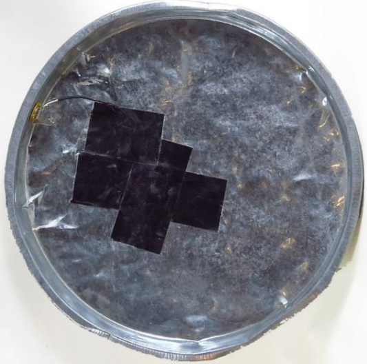
SONICS Noise pan 50mm Piezo on a serving plate for use with amp interaction
