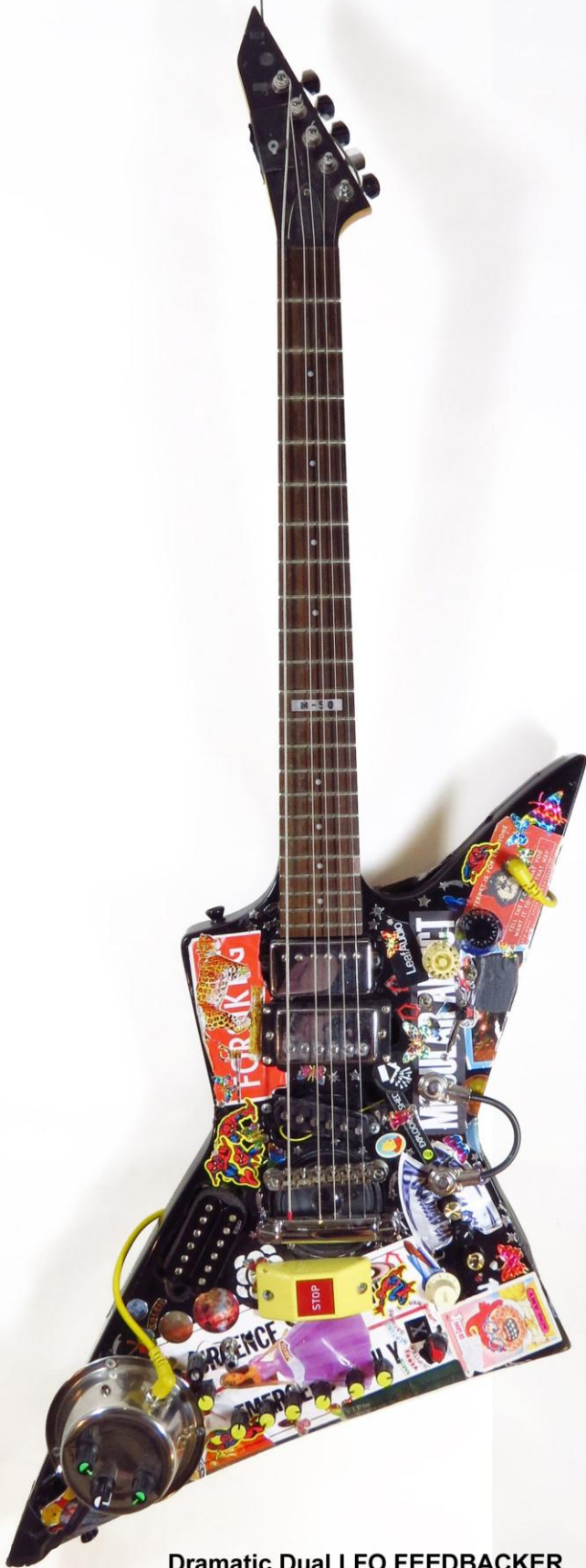
Dramatic Dual LFO FEEDBACKER External input, amp starve, UFO dutch/australian built LFO, homemade LFO intergrated, Stopbutton killswitch, input level blend Base: LTD EX50 neck swap LTD m50 Amplifier: 1W Marshall MS-2 Pickup: Humbucker in neck, humbucker looking single coil inmiddle, single coil bridge,
